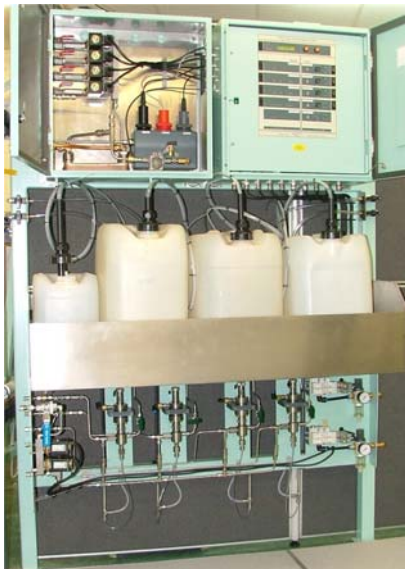
AQ300HP System for feed, condensate and 2 boiler samples (up to 100 bar) shown with 4 high pressure chemical dosing pumps (flooded suction) controlling oxygen scavenger, condensate treatment and a boiler product to each boiler. (External HP coolers not shown) This unit also controls blowdown (up to 100 bar).
