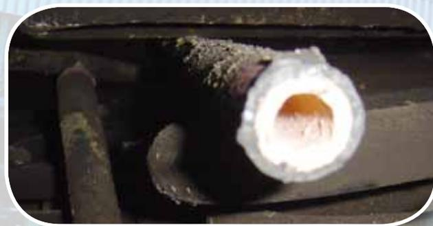
*Above: An example of scaling/chemical blockage inside a heater tube from a watertube boiler.*
