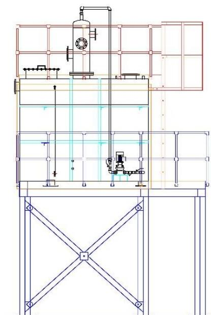
In modern Energy Centres there are no mezzanine floors so to ensure that there is always sufficient static head pressure (NPSH) to prevent boiler feed pump cavitation atmospheric feedtanks have to be elevated high enough to ensure that the normal water level (NWL) provides sufficient static pressure under all operating conditions. The rule of thumb is between 4 and 5 metres above the pump inlet. For the sake of argument let us say that we are catering for a 10,000kg/hr 10 Bar boiler plant.
