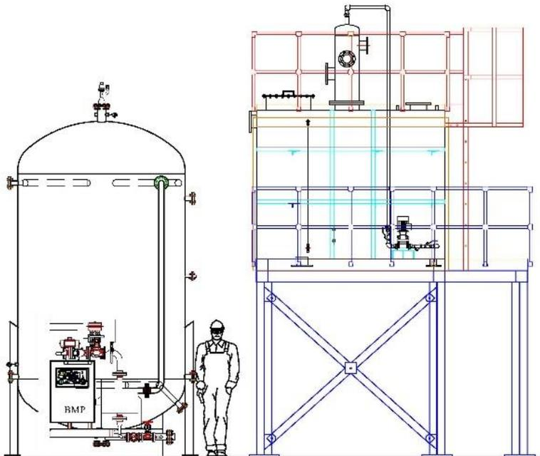
A like-for-like comparison between the existing rectangular tank and support frame and the floor mounted circular vertical tank clearly illustrates that the circular tank design is a cost effective, viable option. Don't forget that the 2m x 2.5m x 2m tank only holds about 7.5m<sup>3</sup> of water compared to the circular tank which holds 10m<sup>3</sup>. But changing the shape of the tank is only part of the answer.
